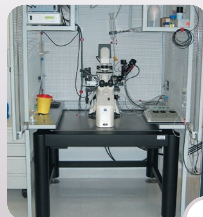
▶ Active Workstation 900 with patch-clamp setup inside a Faraday cage.
